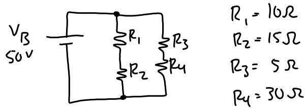
$$\begin{aligned}R_1 &= 10\Omega \\R_2 &= 15\Omega \\R_3 &= 5\Omega \\R_4 &= 30\Omega\end{aligned}$$
