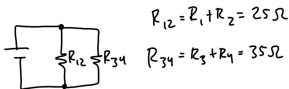
$$V_B \quad \frac{1}{R_{eq}} = \frac{1}{R_{12}} + \frac{1}{R_{34}}$$
